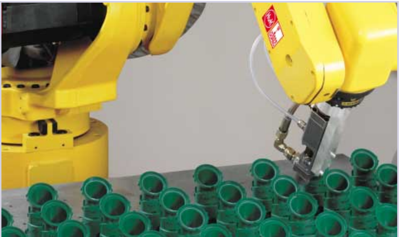
▲ Laying beads of grease as a lifetime lubricant for synthetic swivel joints of vacuum cleaners. Modern metering technique from the Hilger u. Kern / Dopag group in combination with a robot.
