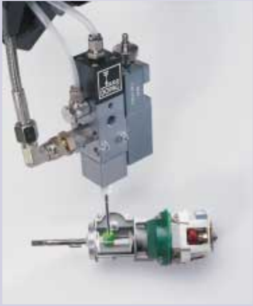
▲ Lifetime lubrication for the drive motor of a vacuum cleaner. The Hilger u. Kern/Dopag group supplied the know-how and the technique.
