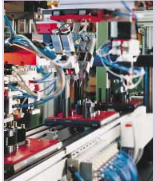
▲ An automatic assembly line for car seats. The Hilger u. Kern / Dopag group supplied the complete grease metering system.
